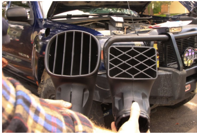
Airflow (left) and Safari (right) air ram designs
