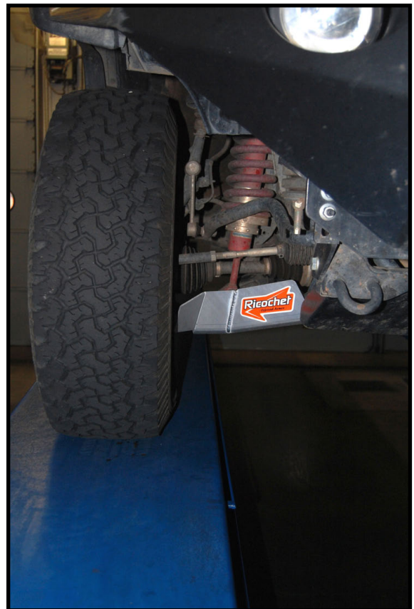
These skids protect one of the lowest hanging areas of the FJ's suspension
